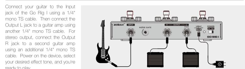
When the battery is low (indicated by the power LED flashing green), use a USB-C to USB-A cable to connect the Go Rig I to a USB power adapter. Once fully charged, the LED will turn green.
