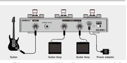
When the battery is low (indicated by the power LED flashing green), use a USB-C to USB-A cable to connect the Go Rig I to a USB power adapter. Once fully charged, the LED will turn green.
